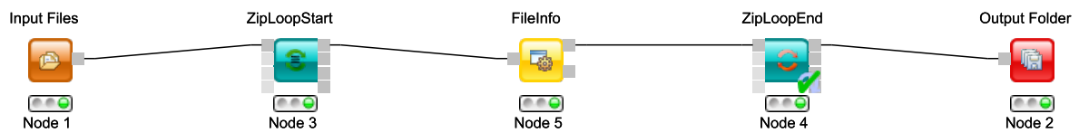
Figure 5: A minimal workflow calling FileInfo on multiple files in a loop.
